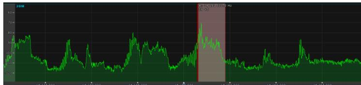
On the left side of the graph of the spectrum analyzer is a vertical scale, which is visible on the power level of signals in the ether. He appears in the levels dBm.
