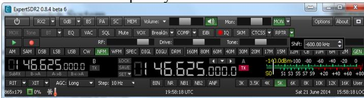
When switching the transmitting frequency shift to work through a repeater sub. the receiver shows the transmitted frequency and the primary receiver displays the received frequency.
