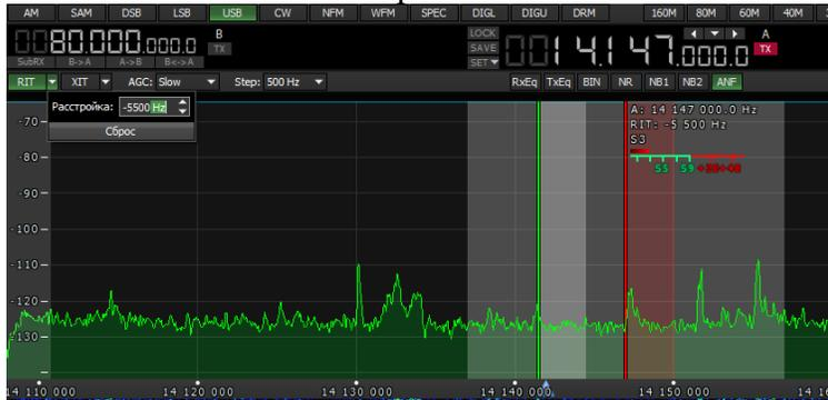
Pressing RIT, the spectrum analyzer graph shows highlighted portion of frequencies of the possible frequency offset and the VFO crosshair settings.
