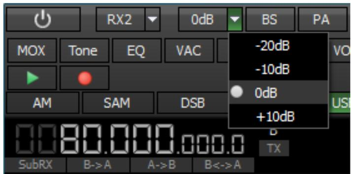
There are 2 levels of attenuation, -10dB and -20dB, and one level of pre-amp gain, 10dB.
